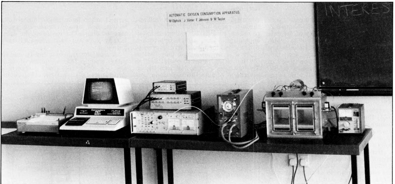
Investigating the effects of environmental temperature on metabolic rate and heat production in small newborn animals (see Fig. 5 and text). Shown are: from left to right: X-Y plotter; 16K PET; (top to bottom) 8-channel DAC unit, 16-channel ADC unit, oxygen valves controller/temperature monitor/oxygen, and CO 2 monitor; oxygen level monitor; dual chamber; power supply.
